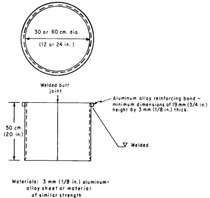
FIG. 1 Infiltrometer Construction
